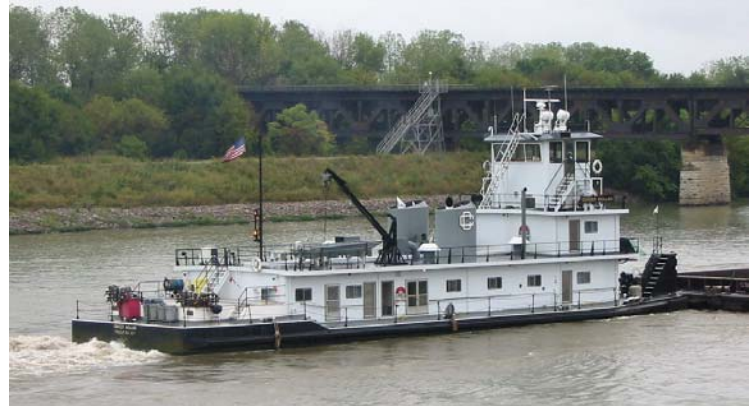
Test vessel M/V Ginger Moller: Length 120 ft. Twin screw fixed pitch: Main engines: Twin EMD 16-645E6 3600 Hp
