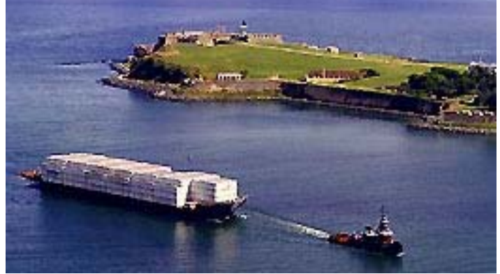
Test vessel M/V Chinook: Length 133 ft. Twin screw fixed pitch: Main engines: Twin EMD 16-645E2 3900 Hp
